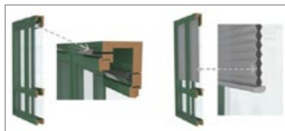
Integration of air supply valves and shading blinds into the double-windows developed for the Budapest case study buildings (Image: NTNU)
